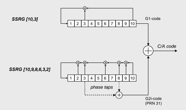
The C/A code generator produces a different 1023 chip sequence for each phase tap setting. The C/A codes are defined for 32 satellite identification numbers (PRN ID).
