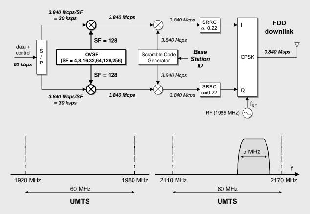
Traffic data (voice) is multiplexed with control information (pilot bits, transmit power control bits, rate information, ...). The serial-to-parallel converter maps the 60 kbps to the I and Q branch of the QPSK modulator. This produces a 30 ksps symbol rate. The I and Q branches are then spread to the 3.840 Mcps chip rate with the same Orthogonal Variable Spreading Factor (OVSF) code. Since the spreaded bandwidth is the same for all users, multiple-rate transmission needs
